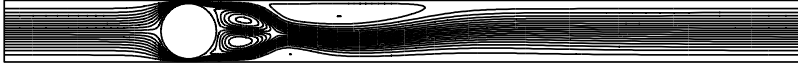
FIGURE 7. Streamlines of the steady asymmetric flow at B=0.9 , \alpha=0 , R=114.3 . Contours of the streamfunction are equally spaced.
